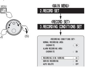
2 Turn the J-dial to select "OVERWRITE" for the normal or the alarm recording area, and then turn the S-dial clockwise.
